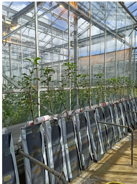
Figure 6. Rhizotrons to assess the effect of dwarfing on RSA in the glasshouse compartment.
