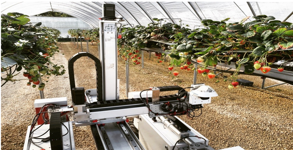
Figure 6: Strawberry harvester mounted on the Thorvald platform harvesting berries using the object detection approaches mentioned above.
