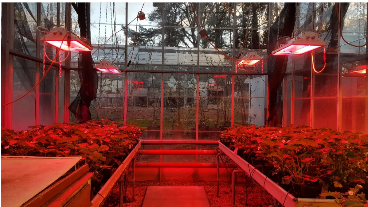
Image 1: Experimental set up of tuneable LED lighting units
